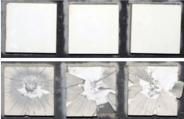
Figure 14: Due to the combination of high adhesive strength and damping performance the targets bonded with silane epoxy are not delaminated.
