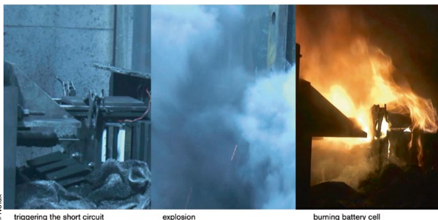
Figure 4 > Battery cell carrier cover in a challenging impact test: Impact/explosion of a 4.2 V Li-OH battery, performed at the Center for Solar Energy and Hydrogen Research in Ulm (Germany)
