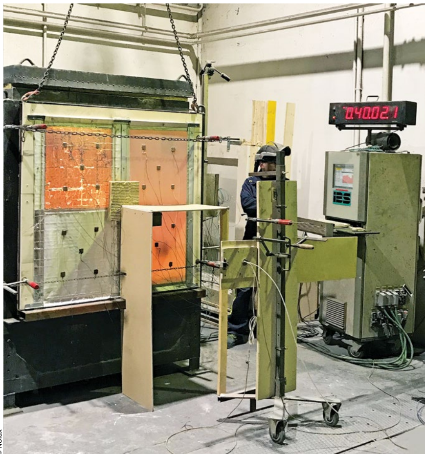
Figure 8 > Fire test according to EN 1634-2019 at the IBS, Linz
