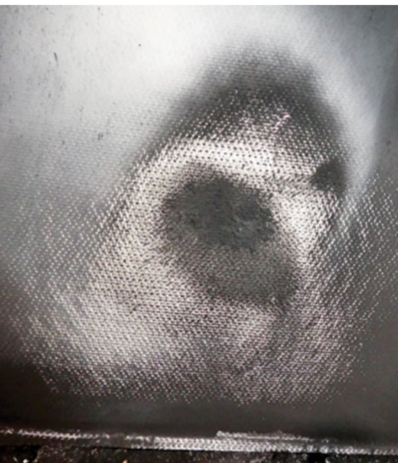
Figure 5 > Impact test at the ZSW, Ulm: Test specimen consisting out of fiberglass fabric coated with a combination of reflective and insulating Nolax/Hearnes products thereafter bonded to an aluminium plate; the impact side shows neither a hole nor a burn through.
