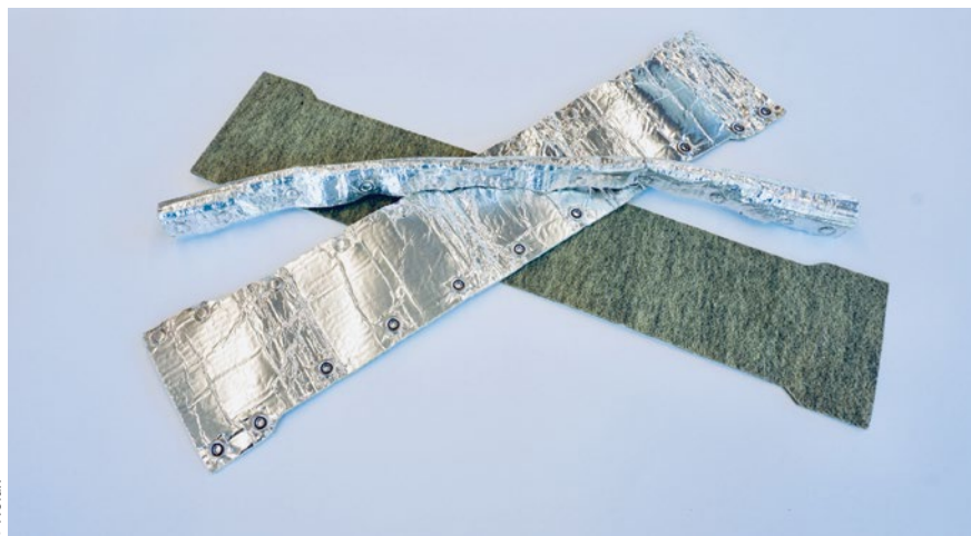
Figure 2 > Flexible material composite for heat protection sleeves for exhaust gas control flap in a truck. Here, temperatures of up to 400 °C must be withstood over the long term.
