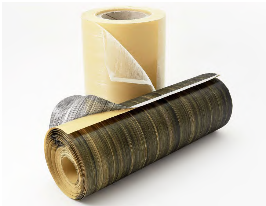
Figure 2 > Fiber-reinforced adhesive films from Nolax. Unidirectionally arranged filaments are embedded in an adhesive and can be processed at elevated temperature and pressure, for example, into membrane sails.
