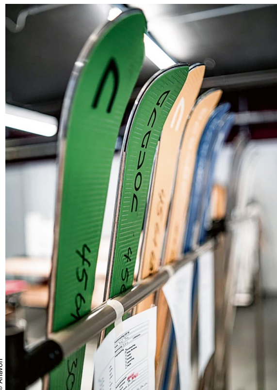
Figure 1 > A typical ski: multi-material laminate of wood, aluminum, steel, and polymers
