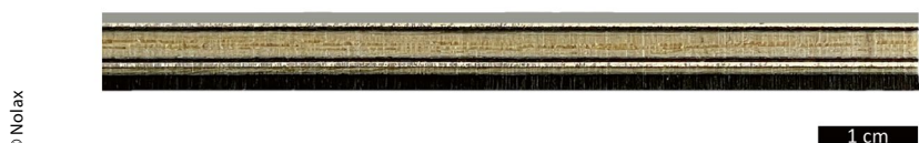
Figure 4 > Cross-section of a multi-material laminate; materials from top to bottom: co-polyamide top sheet, aluminum top chord, neoprene rubber, ash core, neoprene rubber, aluminum bottom chord, ash cut veneer, ultra-high molecular weight polyethylene running surface
